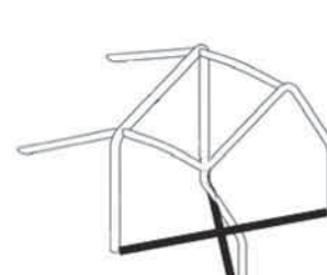
P X brace on floor dwg. 253-31
