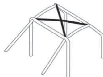
O X brace on roof dwg. 253-12
