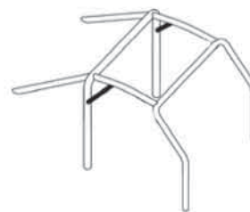
K Rear hoop reinforcements dwg. 253-31
