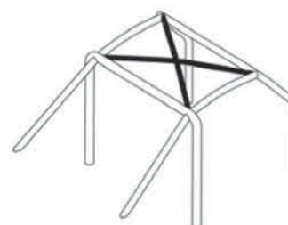
O X brace on roof dwg. 253-12
