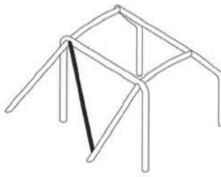
X X diagonal on rear arm dwg. 253-20
