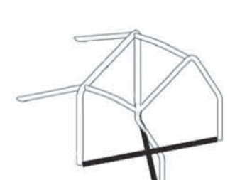
P X brace on floor dwg. 253-31
