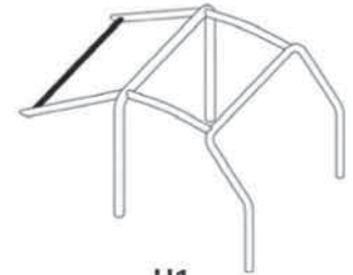
H1 Wrap around harness attachment bar dwg. 253-18
