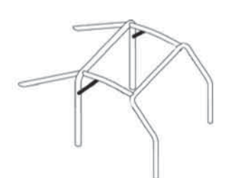
K Rear hoop reinforcements dwg. 253-31
